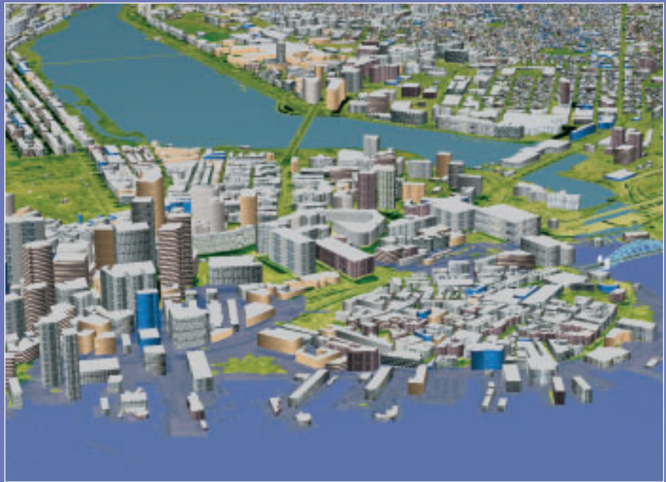
"Effects of a 100-year coastal storm surge in Boston with sea level rise by 2075. This computer graphic shows the floodplain in 2075 with Boston harbor in the foreground and the Charles River in the background."
