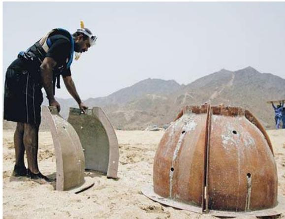
**Figure 5-** *Molds for artificial reef structures*
